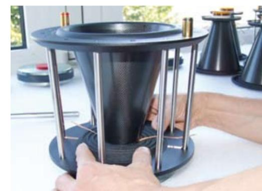
Above: The DDD is not centred until shortly before it is finished. This is partly done by hand.
