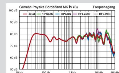
For an omni-directional bending wave transducer the frequency response of the Borderland is very good. The bass looks just as good as it sounds: reaching extremely deep. The drop-off at 15K due to the principle used is not audible. The purple and green curve show the effect of the level jumper: subtle and primarily in the range around 10kHz.
