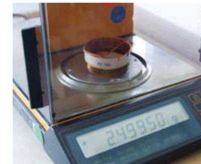
Above: The DDD voice coil on the precision scales. Below: This crossover network is assigned only to the bass.
