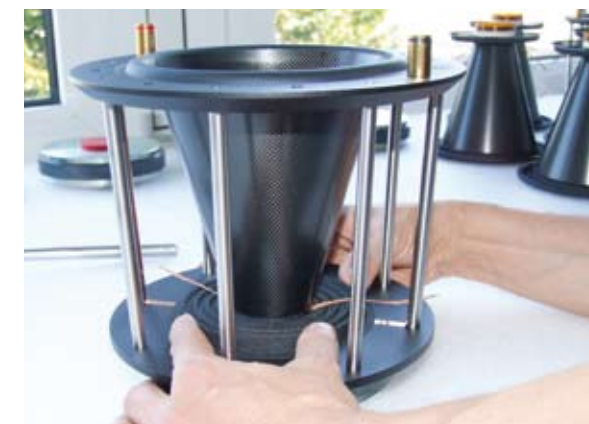
Above: The DDD is not centred until shortly before it is finished. This is partly done by hand.
