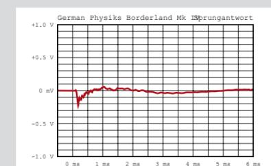
A model example of impulse precision: while the reproducing step signal is inverted, it is on the other hand steep-flanked and time-correct with a single step, as with a wide bandwidth system. After brief transient oscillation the system very quickly comes back to rest. No stereo exaggeration and no resonance cloud the faultless image.
