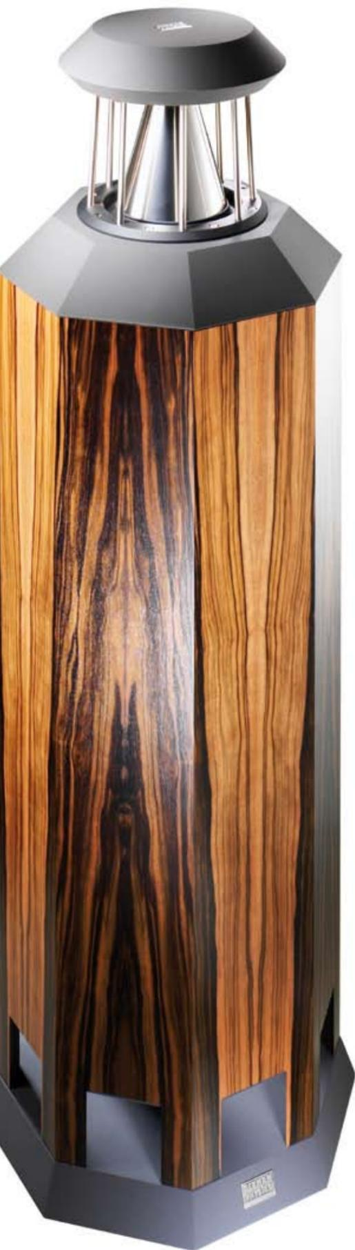
a Helmholtz resonator, which dampens the vertical standing wave at 240 hertz. Although the bass already bails out at 150 hertz, this buzzing frequency would nevertheless be irritating.
